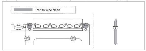
**3** Load the detection pin in the ATC magazine's number 6 position.
