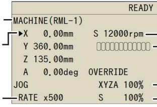
The value displayed here is the currently set spindle rotation speed with the override taken into account.
