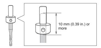
3 Use the hexagonal screwdriver to secure the mounting screw.
