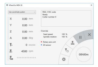
VPanel is an application that can be used to operate this cutting machine from a computer screen. It has functions for outputting cutting data, performing maintenance, and making various corrections. It also displays information such as the cutting machine status and errors.
