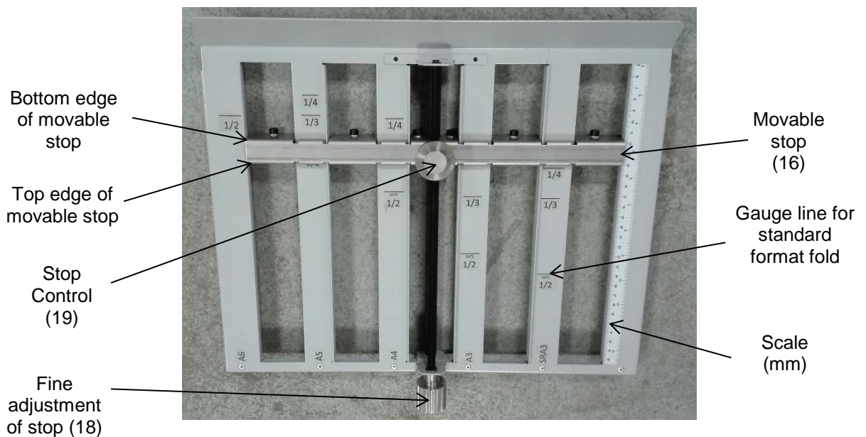
Fig. 4: Bottom fold plate - 3 mm (and 6 mm) clearance
