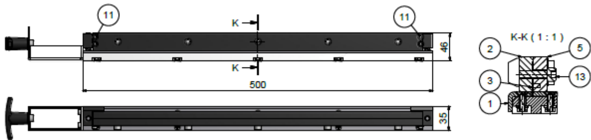
Fig. 5: Perforating tool 2:1- 9 TPI (571 40 465a) – standard equipment. Micro perforating tool (571 40 464) as optional accessory.
