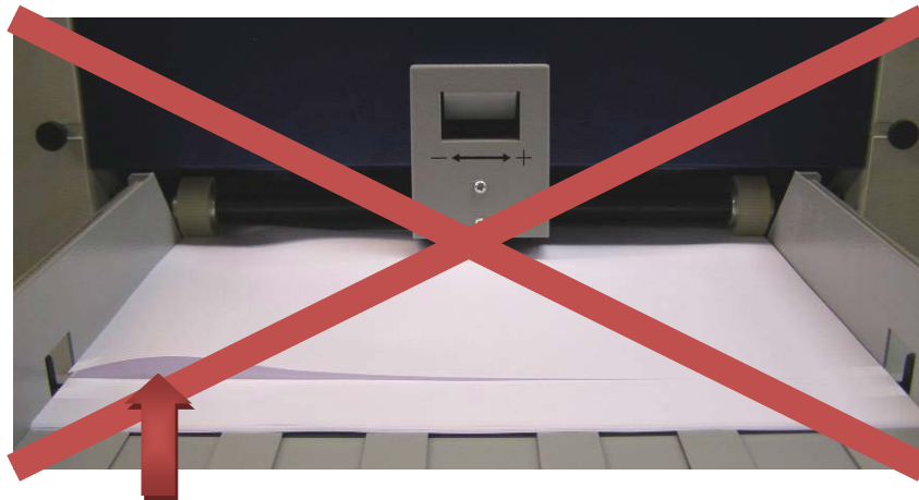
Fig. 16: Example of incorrect setting of table thrust – too much thrust for the low paper grammage
