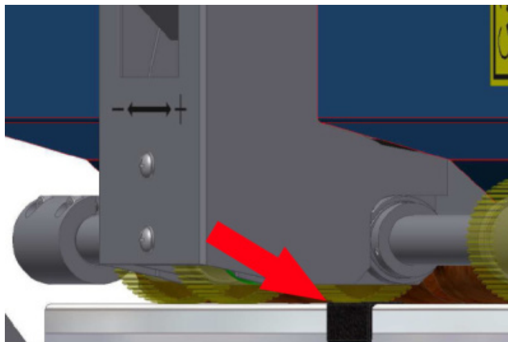
Fig. 35: The gap between feeding wheel and separator must be 0,05 – 0,1 mm wide.
